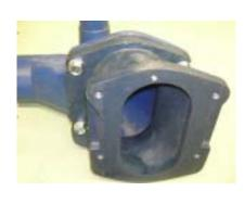
4. Using (4) of the offset's bolts (\*or the remaining two), secure the offset to the fitting, making sure that all of the bolts are threaded tight. The bolts should thread through the slots of the offset and the holes of the gasket and fitting.
